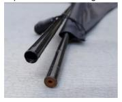
a car than when flying. The Prism Ozone in the pictures above had several failures to the tubes of its lower spreader, which only stopped when the kite was kept in a drainpipe during transport rather than just in the bag that was supplied with it. The second weakness has so-far only been seen with the Skyshark Zero tubes used in the writer's Skyburner Ocius SUL, and that is that the walls at the narrower end of the tapered tubes are so thin that they fray during repeated
