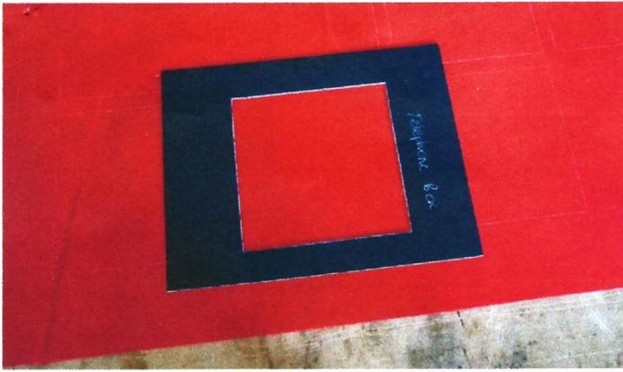
In the kit you will find a piece of card with a hole cut in it. This hole is the same size as each window and is your template. Place this down on the face of the kite so that a marked window is framed. Using your hot knife cut round the inside of this template. Lift the cut section away then move the template to the next window and repeat until all the windows are cut out. (Alternatively use a metal rule and cut round each window that way being careful not to go past the marks)
