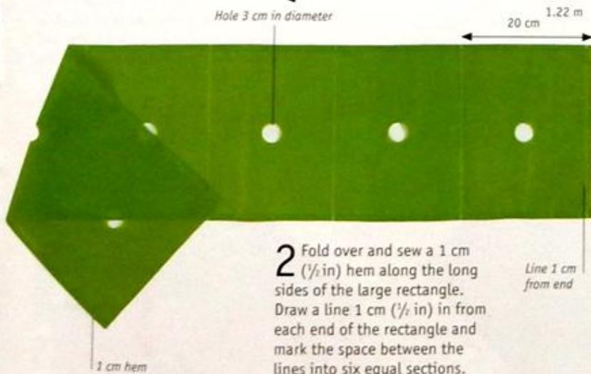
**2** Fold over and sew a 1 cm (1/2 in) hem along the long sides of the large rectangle. Draw a line 1 cm (1/2 in) in from each end of the rectangle and mark the space between the lines into six equal sections. Cut a circular hole in the centre of each section.
