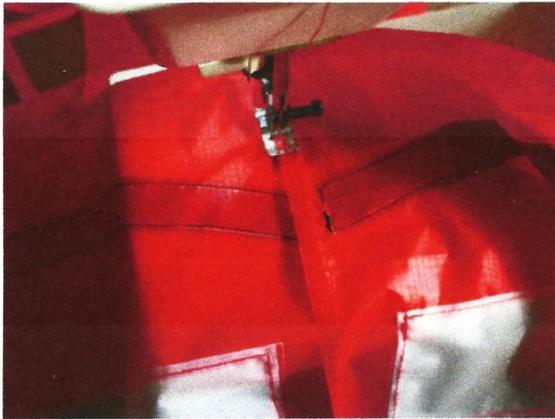
Put two panels face to face and match the top edges. Sew 1cm in from the edge to join the two. At the marked halfway point place the 6cm tab (lower bridle point) between the two panels, folded edge in, with the ends level with the edges. Sew, reverse then sew on down to the bottom of the kite. Open the panels out face down. Fold over the 1cm seam and sew it flat from the top to the bottom of the kite.
