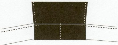
Insert the one end of the 2mm carbon spar (approx. 1.7m long) and feed round the entire sleeve then cut so that the spar ends are either side of the sewn middle section of the dacron. End caps can be added.
