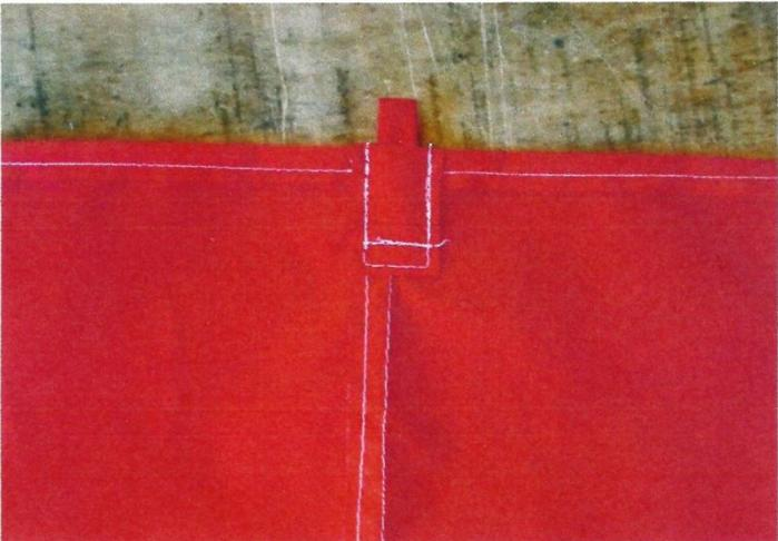
Finally, take an 8cm tab. Fold in half and feed the ends between the pocket and the kite only on the pocket on the edge that has the bridle point at the halfway mark. Sew in as shown on photo left.
