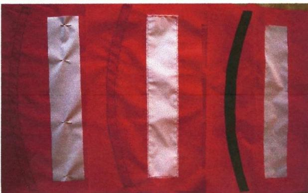
You can see all three stages here from pinning, through sewing to cutting away the red on the face of the kite to leave white panel showing.
